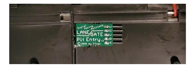
5. Locate the red wire shown below and gently pull its spring clip out of the track rail. Cut off the clip, then use wire strippers to remove 4mm of insulation from the end of the wire.
