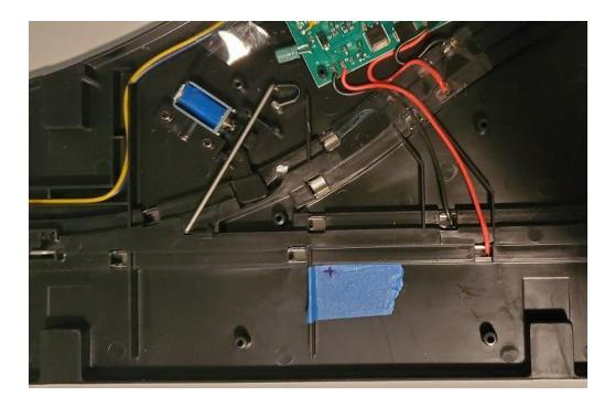
3. Using a 2mm or 1/16" bit, drill a hole on the mark you made. Remove the masking tape after drilling.
