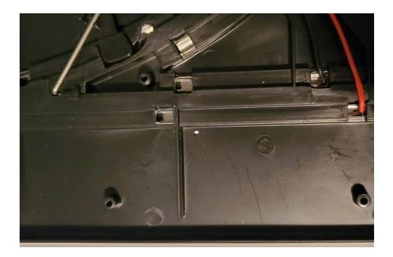
4. Low-temp hot glue is the preferred method of mounting the PEN board. Be sure to put a dab over the hole to act as a lens and keep debris out. Go easy with the glue at first. Once you are sure the LED is aligned with the hole, you can add more glue later.
