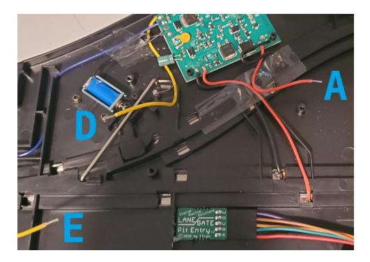
11. Secure wiring with tape or hot glue. Leave a gap between the yellow wire and rail #4.
