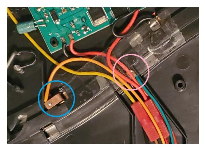
10. Make connections for "A", "D", and "E" using Posi-lock splices.
