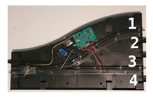
8. The color of the wires in the 5-wire pigtail of the Lane Gate Pit Entry is random. The important detail of each wire is its position/letter (A-E), which is printed on the edge of the Lane Gate board.
