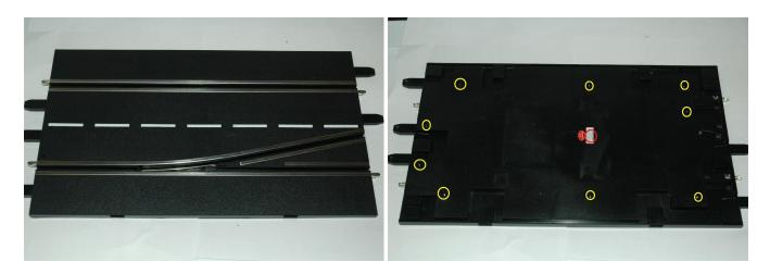
7. Rotate the section so that the IR sensor (with blue/yellow wires) is at bottom right. The numbers on the right side of the picture help identify each of the track rails. The factory red (+) wire may be located in rail #1 or #3 and either position is acceptable. The factory black (-) wire must go to rail #4. If it is currently attached to rail #2, move it to rail #4.
