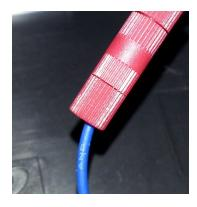
Tighten the end and pull gently on the wire to verify it is secure.
