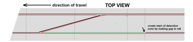
16. When you add anti-collision to lane changers, it becomes important to have power taps in the right places. A power tap to the isolated rail inside of the detection zone will defeat the anti-collision circuit. Likewise, creating the isolated rail means the track is no longer a continuous loop, so power taps/jumpers will most likely be needed in some spots.
