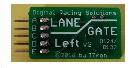
The DRS Lane Gate "Left" chip is for Carrera D124/D32 lane changers where cars can move from the right lane to the left lane only. That includes models #30343 Straight Type, #30363 Left Curve - Out to In, and #30364 Right Curve - In to Out.
