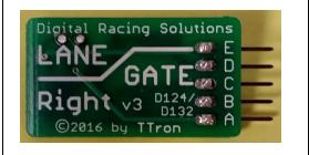
The DRS Lane Gate "Right" chip is for D124/D132 lane changers where cars can move from the left lane to the right lane only. That includes models #30345 Straight Type, #30362 Left Curve - In to Out, and #30365 Right Curve - Out to In
