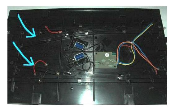
3. The numbers on the right side of the picture help identify each of the track rails. The factory red (+) wire needs to be located in rail #1. If it is in rail #3, move it to #1. The factory black (-) wire must go to rail #4. If it is in rail #2, move it to rail #4. In the image below, both of these wires need to be moved.
