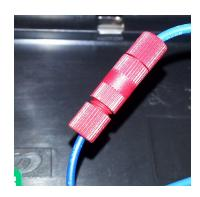
Push the bare wire into the end until it stops.
