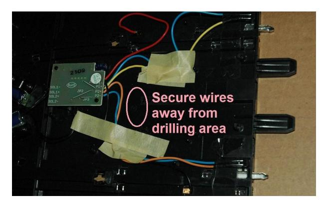
Measure, mark, and drill from the top of the track. Use 3mm or 7/64" drill bit. End result should look like:
