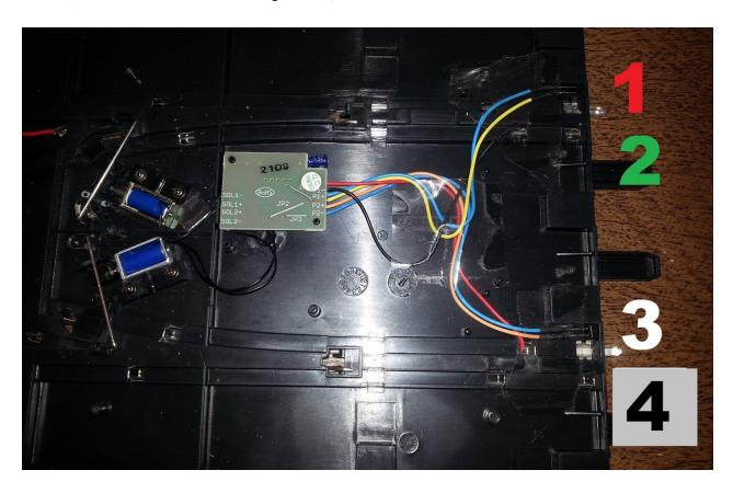
4. The Lane Gate Double will mount between the lanes. Examine your track section and cover plate for ribs, posts, or flanges that might restrict where you will locate the chip. You'll be drilling two small holes near the centerline of the track. For the sections we've seen, a good location is 83mm (3.25") from the end. Secure all wiring away from the hole locations as shown. This picture also shows the red and black wires from step 3 now moved to the proper rails.
