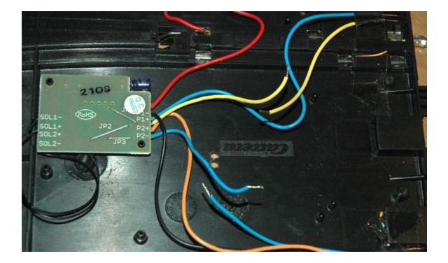
6. The color of the wires in the 8-wire pigtail of the Lane Gate Double is random. The important detail of each wire is its position/letter (A-H), which is printed on the edge of the Lane Gate board.
