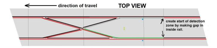
12. When you add anti-collision to lane changers, it becomes important to have power taps in the right places. A power tap to the isolated rails inside of the detection zone will defeat the anti-collision circuit. Likewise, creating the isolated rails means the track is no longer a continuous loop, so power taps/jumpers will be most likely be needed in some spots.
