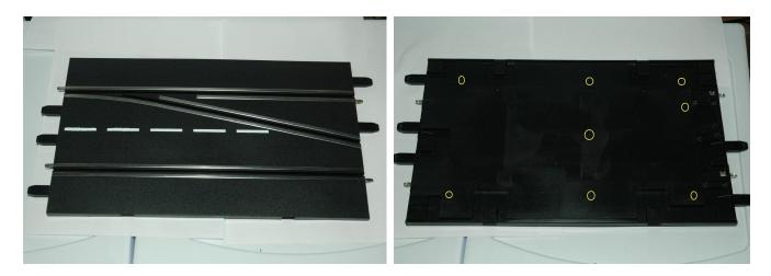
3. Isolate the short inside rail by removing the jumper wire as shown. It is <u>usually</u> a red wire.
