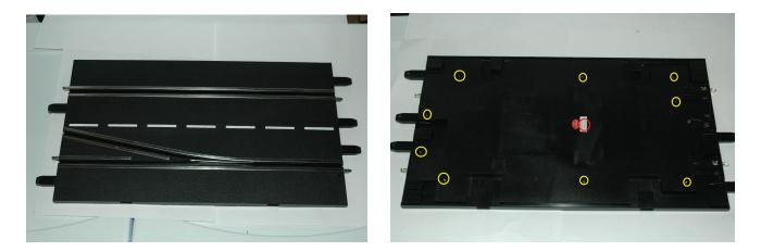
7. Place the section so that the IR sensor (with blue/yellow wires) is at top right. The numbers on the right side of the picture help identify each of the track rails. The factory red (+) wire must go to rail #1. If it is currently attached to rail #3 (as shown in picture), move it to rail #1. The factory black (-) wire may be located rail #2 or #4 and either position is acceptable.
