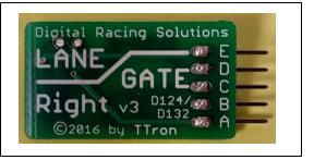
The DRS Lane Gate "Right" chip is for D124/D132 lane changers where cars can move from the left lane to the right lane only. That includes models #30345 Straight Type, #30362 Left Curve - In to Out, and #30365 Right Curve - Out to In
