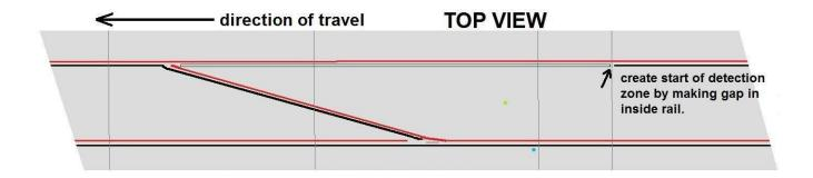
16. When you add anti-collision to lane changers, it becomes important to have power taps in the necessary places. A power tap to the isolated rail inside of the detection zone will defeat the anti-collision circuit. Likewise, creating the isolated rail means the track is no longer a continuous loop, so power taps/jumpers will be most likely be needed in some spots.
